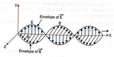
(b) The speed of electromagnetic wave  $|c| = \frac{|E_0|}{|B_0|}$
